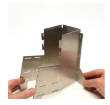
**Step 2**Orient the <u>Floor Plate</u> as shown and slip into the bottom slots of the side plate on the left. Be sure to position it so the smaller tabs are on the left as shown. (Do not engage with the right side plate yet).
